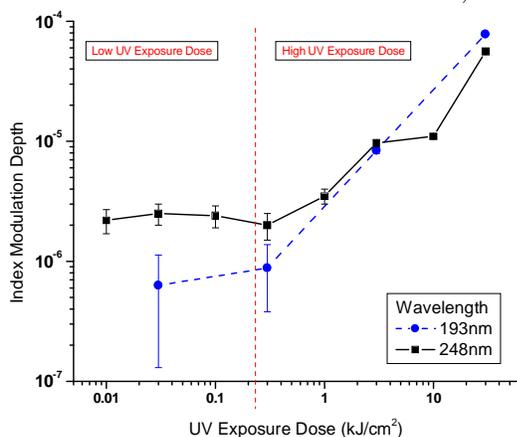
Fig. 1. Refractive index modulation depth as a function of dose.
