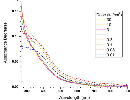
Fig. 4. Absorption decrease caused by thermal annealing at 200°C
