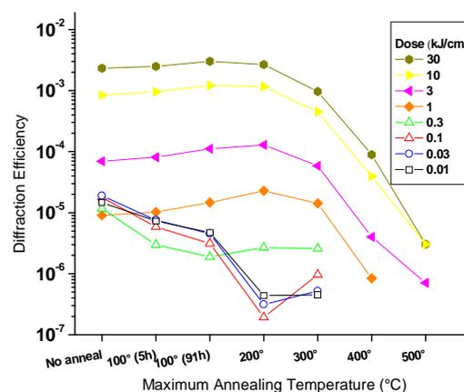
Fig. 2. Grating diffraction efficiency as a function of annealing.
