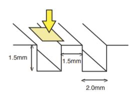
Diamond #600 (Metal Bond) Wheel dia 100mm (2400 rpm) Machine speed 4mm/min
